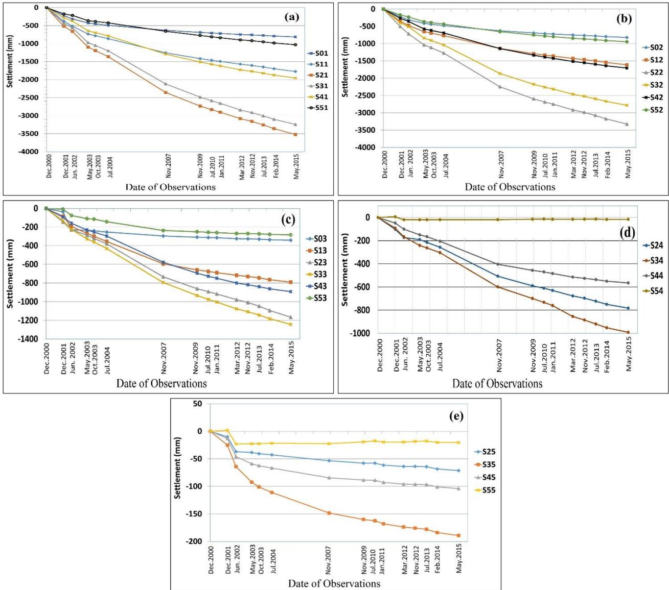
Figure 4. Settlement of target points of the Masjed-Soleyman dam derived from 15 sets of terrestrial geodetic measurements; (a) points of the upstream edge of crest, (b) points of downstream edge of the crest; (c) & (d) and (e) points installed on the downstream slope at elevations of 347 m, 310 m, and 270 m, respectively.
