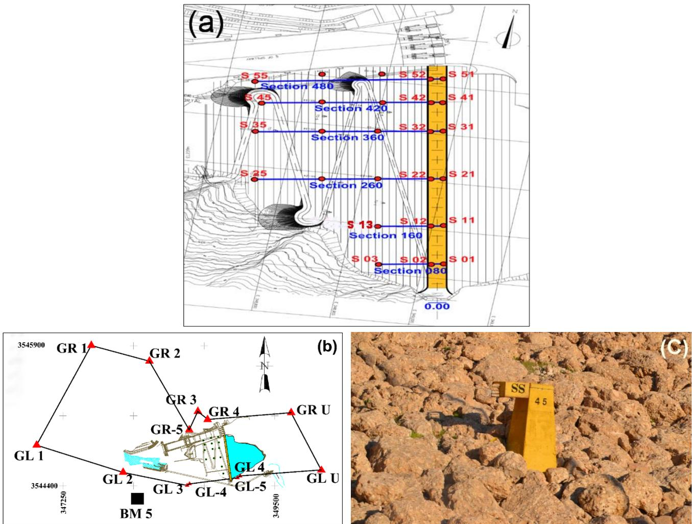
Figure 3. (a) On-dam geodetic network of the Masjed-Soleyman dam. Twenty-six target points were installed on the crest and downstream slope of the dam. The blue lines show the cross-sections of the dam. (b) Off-dam and On-dam geodetic networks: GR3 and BM5 are the fixed points for horizontal and vertical measurements, respectively. (c) Concrete pillar of the geodetic networks established on the dam body.
