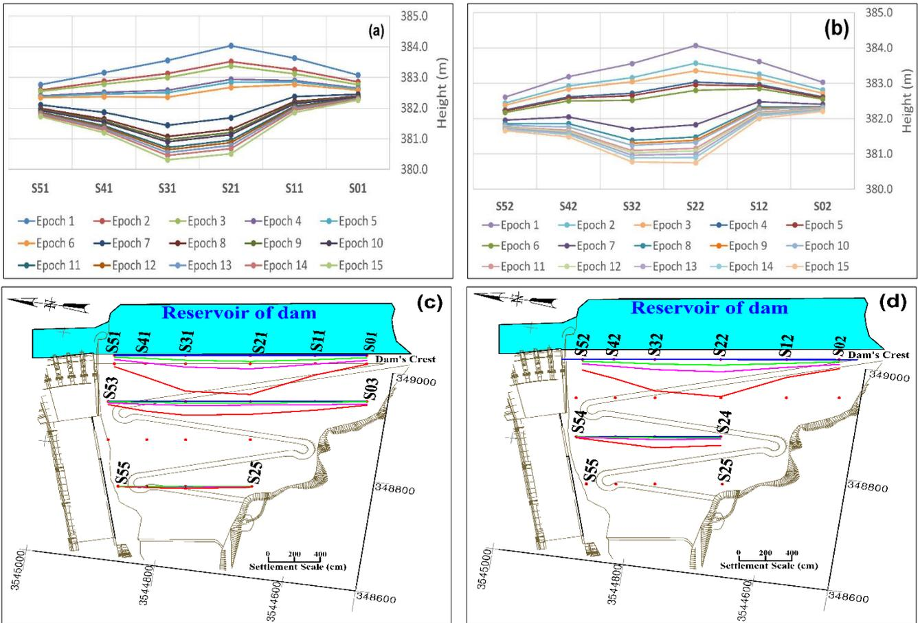
Figure 5. Changes in the heights of the points located on the crest points during 15 terrestrial observations. (a) Upstream edge of the crest; (b) downstream edge of crest; (c & d) settlement of points during three steps of dam operation: 1<sup>st</sup> year (green line), 3<sup>rd</sup> year (magenta line), and 15<sup>th</sup> year (red line) after impoundment of the dam.
