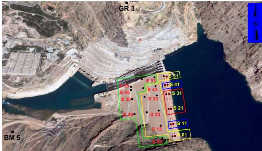
Figure 10. Four zones of settlement in the Masjed-Soleyman dam. Green, yellow, blue, and red blocks represent the zones 1, 2, 3, and 4, respectively. The red block (zone 4) represents the maximum settlement, and the green block (zone 1) represents the minimum settlement of points.
