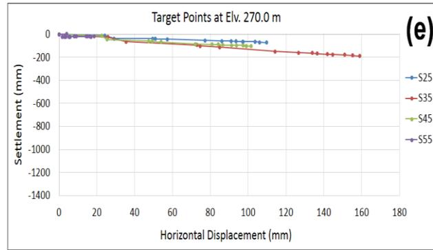
Figure 6. Vertical /horizontal displacement of target points located on the crest and downstream slope of the dam. (a), (b) displacement of points installed on the upstream and downstream edge of crest, respectively. (c), (d) and (e) show the displacement for points located at the downstream slope in elevation of 350 m, 310 m, and 270 m of the dam embankment, respectively.
