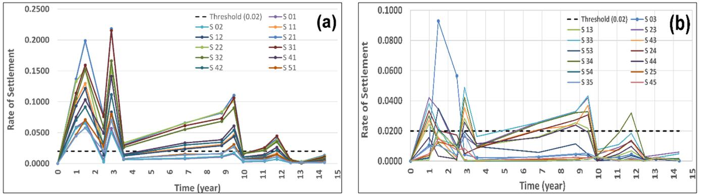
Figure 9. The annual rate of settlement for points of the on-dam network; a) crest points; b) points installed on the downstream embankment of the dam. The Dashed line shows the threshold limit of 0.02 %.
