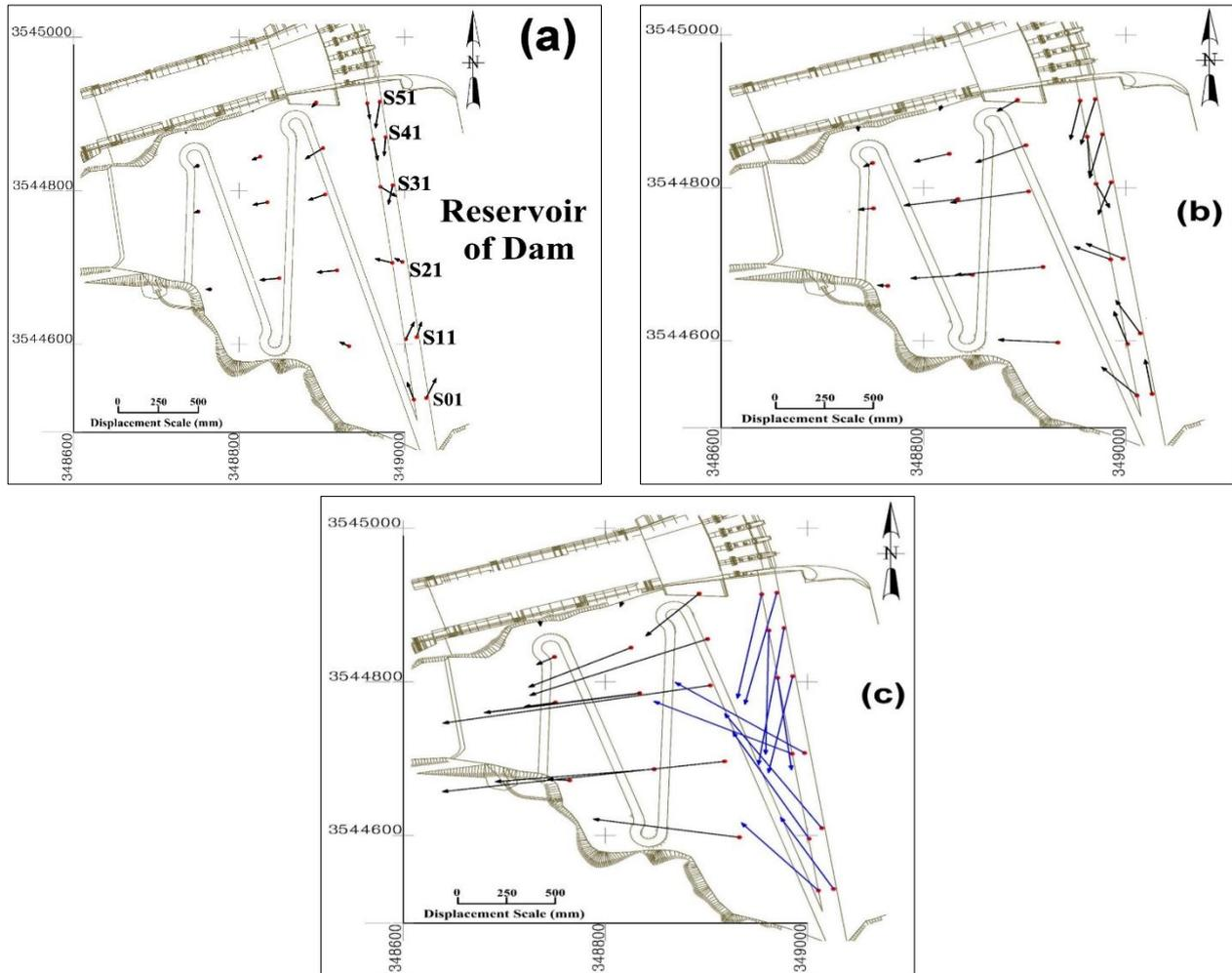
Figure 7. The horizontal displacement of object points installed on dam body; (a) during the first year of dam impoundment, (b) three years after the dam operation, (c) after the 15<sup>th</sup> year of dam operation.
