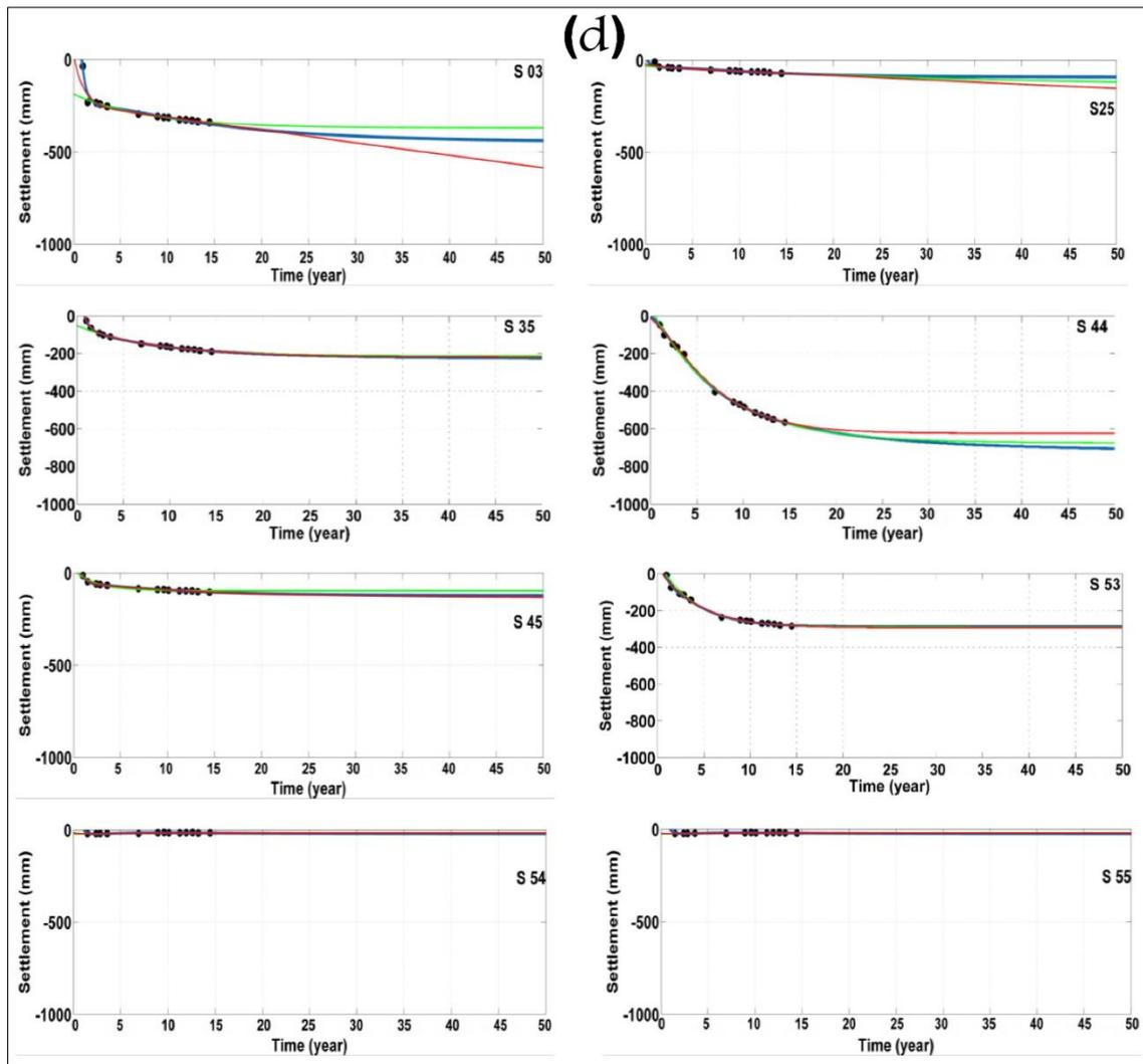
Figure 11. (a-d) Time series of the settlement of object points installed on the dam body during operation by use of 15 years surveying dataset from 2000 to 2015 and relaxation model for prediction of vertical displacement of the dam until 2050: (a-d) for the zones 4 up to 1, respectively.
