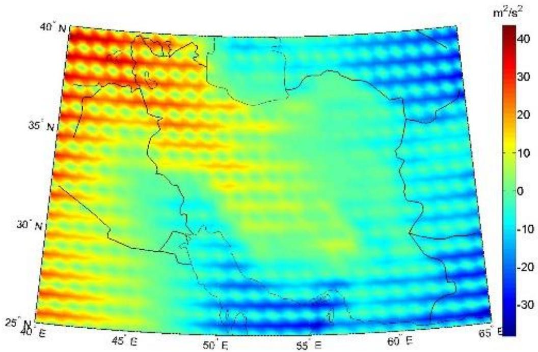
Figure 4: Difference between actual grid, produced by ellipsoidal potential formula, and those derived from interpolation of potential values,  $0.5^{\circ} \times 0.5^{\circ}$  grid
