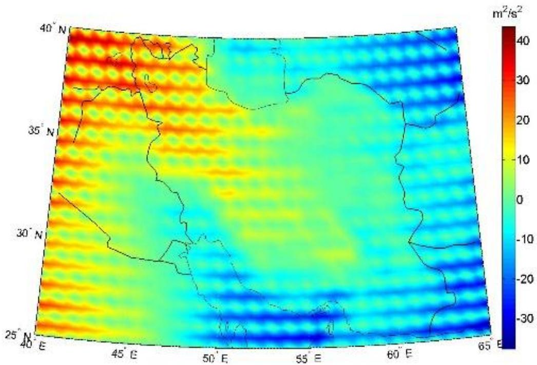
Figure 5: Difference between actual grid, produced by ellipsoidal potential formula, and those derived from the interpolation of potential values by spherical splines,  $0.5^{\circ} \times 0.5^{\circ}$  grid
