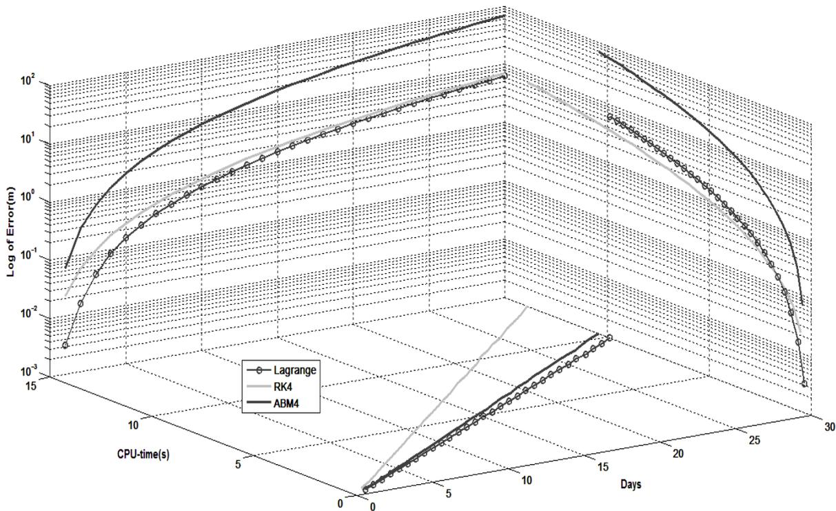
Figure 2. The comparison of the numerical integrations and Lagrange error versus CPU-time in a one-month span.
