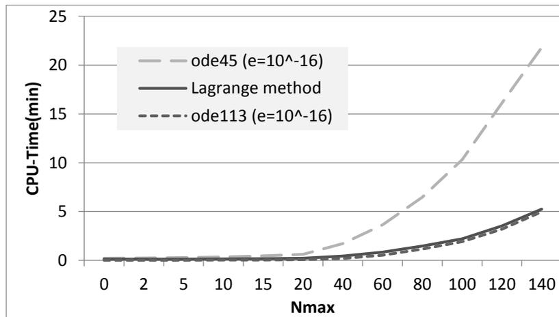
Figure 4. The computation time needed for propagating over one day of the GRACE A satellite using ode45, ode113, and the Lagrange method
