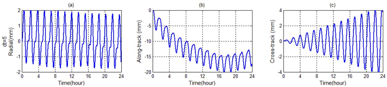
Figure 5. The difference between the reference and Lagrange orbits for Spot 6 satellite with  $dt=5s$  over one day
