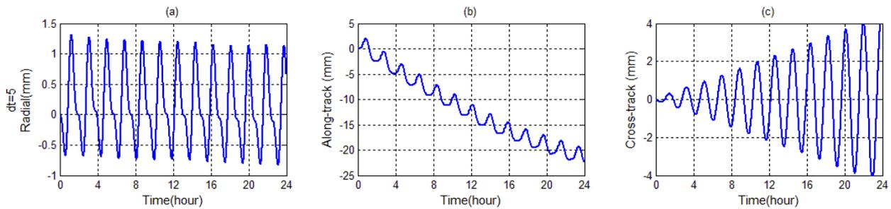
Figure 6. The difference between the reference and Lagrange orbits for TOPEX-Poseidon satellite with  $dt=5s$  over one day
