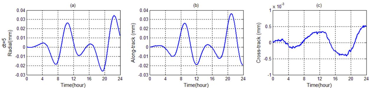
Figure 7. The difference between the reference and Lagrange orbits for GPS 01 satellite with  $dt=5s$  over one day
