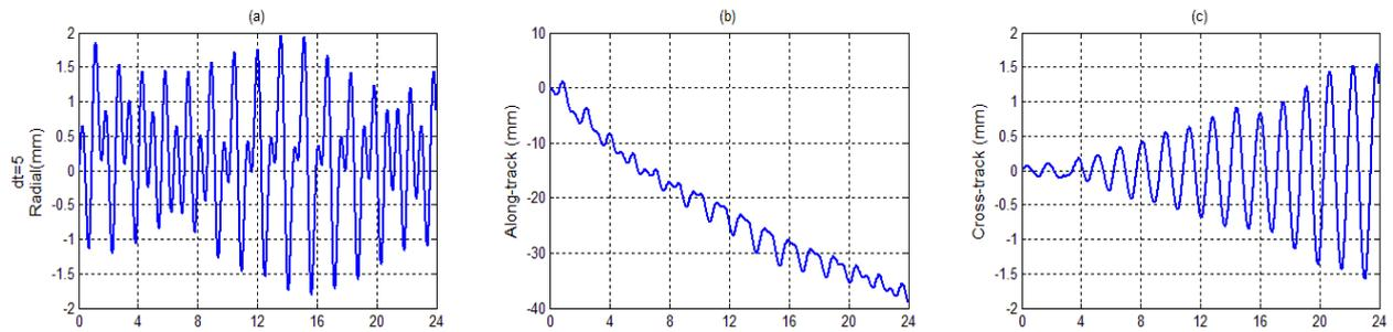
Figure 3. The difference between the reference and Lagrange orbits for GRACE A satellite over one day
