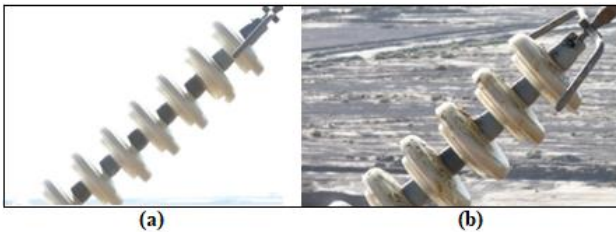
Figure 1 illustrates the difference between a clean and bird-contaminated insulator.
