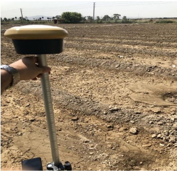
Figure 3.a. The topography mapping using Raimond GPS
