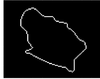
Figure 9. A binary mask illustrating the defined neighborhood (one-pixel-wide strip around the cloudy area) for Scenario 1, applied in the IDW interpolation process for cloud-covered pixels
