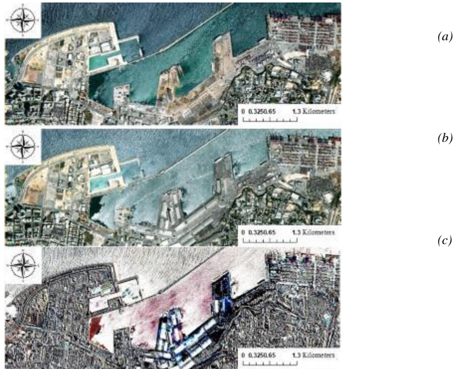
Figure 5: Beirut explosion (a) post-event and (b) pre-event. (c) absolute difference image of spectral values.
